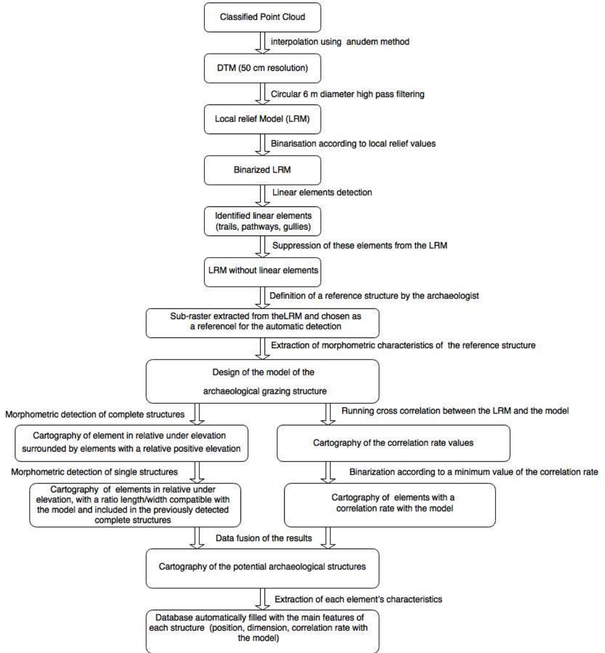
Fig. 5. Flowchart of the approach implemented for the automatic detection process
